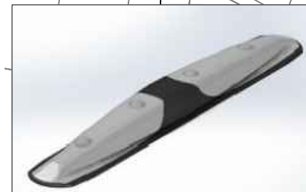
DETAIL 3: CYCLE LANE SEPARATOR 120mm WIDE x 720mm LONG (TYPICAL ARRANGEMENT)
